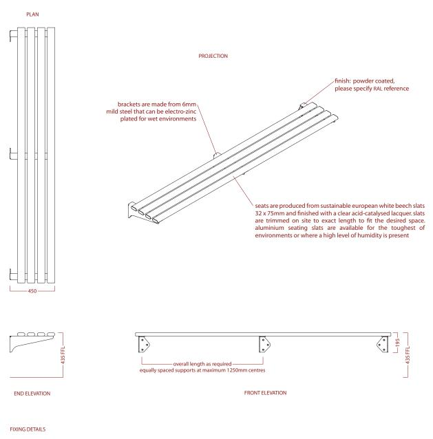
Binns recommended fixing for this unit is Hilti HRD-UGT 10x80 / 10, No 3 fixings per frame. A J Binns can supply fixings as an extra.
