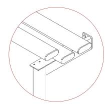
for shorter, non standard lengths a radiussed end has to be applied to the cut
